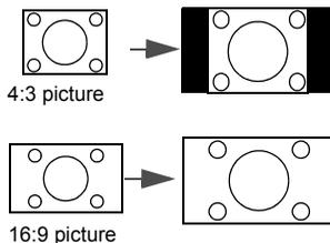
2. **Real:** The image is projected as its original resolution, and resized to fit within the display area. For input signals with lower resolutions, the projected image will display smaller than if resized to full screen. You could adjust the zoom setting or move the projector towards the screen to increase the image size if necessary. You may also need to refocus the projector after making these adjustments.
