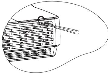
3. Remove the lamp cover by (a) sliding the cover toward the side of the projector and (b) lifting it off.
