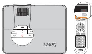
2. Press **Power** a second time. The **POWER indicator light** flashes red, the projection lamp shuts down, and the fans will continue to run for approximately 90 seconds to cool down the projector.
