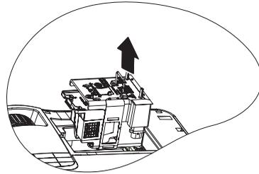
6. Insert the new lamp into the lamp compartment and make sure it fits in the projector.
