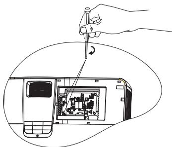
9. Replace the lamp cover by sliding it into place.
