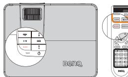
You can set the blank time in the **SYSTEM SETUP > Operation Settings > Blank Timer** menu to let the projector return the image automatically after a period of time when there is no action taken on the blank screen. The length of time can be set from 5 to 30 minutes in 5-minute increments.
